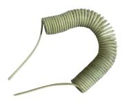
This very special spiral earthing cable has been developed for potential equalisation (earth connection). A fine-stranded earth wire (yellow-green) is guided loosely in a transparent polyurethane hose. This product is designed to fulfil the highest safety requirements and to be ready for use under extreme conditions.
