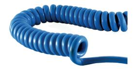
The PVC/PUR spiral cables are suitable for special applications in control, measurement and regulation technology in intrinsically safe systems. The concentric stranding with static shielding prevents interference in the transmission area. The poly-fleece banding guarantees optimum, 100% shielding at low and medium frequencies and filters external electrical interference.
